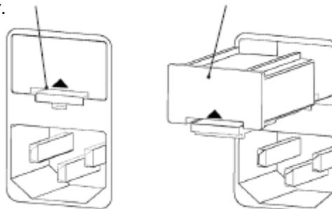
**Important!** Fuses protect equipment by disconnecting loads too large for the circuit design. Always replace fuses with those that conform to the specified fuse rating.
