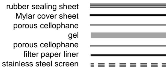
**Note:** Cellophane provides a transparent support for densitometric scanning. Remove all air pockets at every step of this procedure to avoid scanning distortions.
