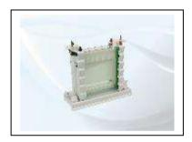
8. Transfer the running module to the gel tank. Fill the inner and outer buffer chambers before loading samples.
