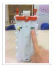
4. Once the green sliding gel clamp is removed the running module is ready to accept the thinner yellow sliding gel clamps for 2-gel sandwiches, either side of the running module, to convert the system to a 4-gel configuration.
