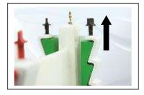
3. Insert a gel cassette into each side of the inner buffer chamber in the running module, and begin tightening the vertical screw-pins.
