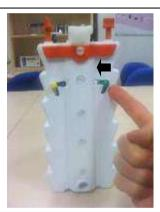
3. Push the green sliding gel clamp out of the running module by gently pressing the protruding pin as shown.
