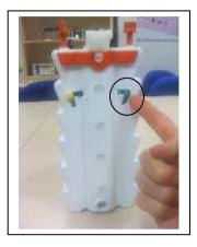
2. Gently push the green sliding clamp horizontally towards the core of running module until it can move no further.
