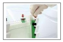
5. Check the bottom of the glass plates to ensure that they are flush together, and place the running module on the casting base; make sure that the cams are facing downwards.
