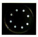
Precision positioning of discs equally spaces on 54mm circle
