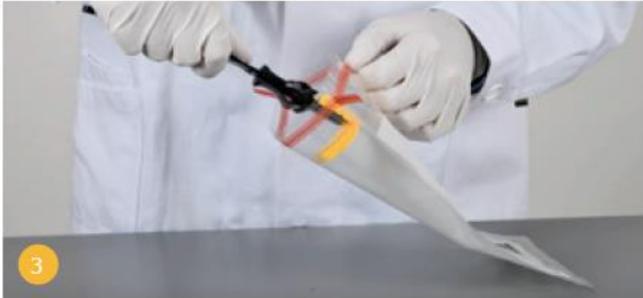
Release sponge from the quick release handle into the Twirl-Tie™ bag provided, by pulling the clip back.
