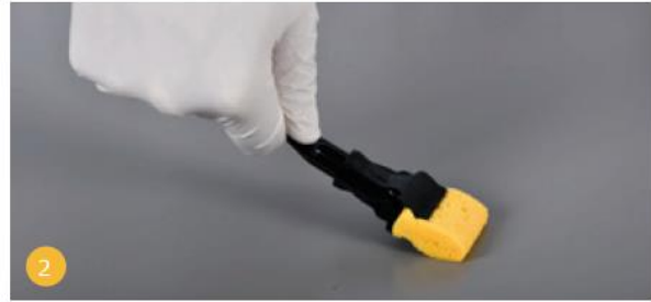
Collect sample by vigorously rubbing sponge on target area (e.g. 30 x 30 cm, 1 x 1 ft.).
