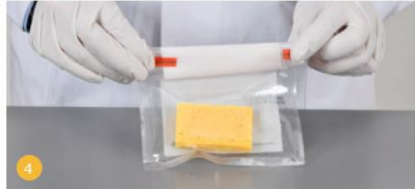
Close the Twirl-Tie™ bag with the wires attached and label it. No switching of gloves between sampling sites needed.
