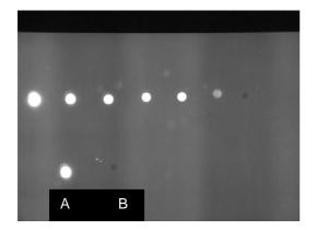
The picture shows a saran wrap with spots of decreasing concentrations of EtBr on a UV transilluminator. On the upper lane 5, 1, 0.5, 0.25, 0.1, 0.05 and 0  $\mu$ g EtBr/ml TAE solutions were mixed with equal volumes of pBS in TE (15  $\mu$ l each). Below a 2  $\mu$ g/ml EtBr containing sample (A, left spot) was decontaminated – the BondEx flow-through contains no detectable EtBr (B, right spot).
