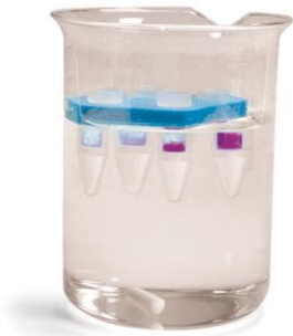
C: Dialysis of the restriction enzyme Pst I in enzyme buffer/8 M urea against pure enzyme buffer
