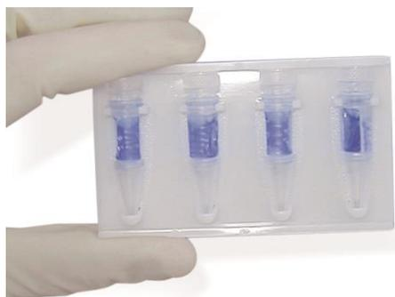
B: ROTI®Elution Tubes MIDI positioned in ROTI® Elution Tube Tray
