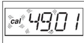
The default setting is 10.00 for a 10 ml device, 20.00 for a 20 ml device and 50.00 for a 50 ml device. The calibration factors may be set between 9.00 and 10.99 for a 10 ml device, between 18.00 and 21.99 for a 20 ml device and between 45.00 and 54.99 for a 50 ml device. Pressing the right key modifies the actual decimal position flashing at the time. When the left key is pressed the device switches to the next decimal position.
