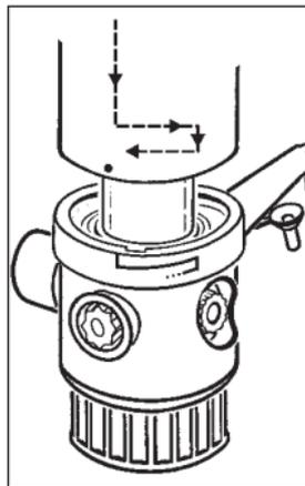
For assembly, align the toothed rack in such a way, that the teeth face the view glass. Then turn the hand wheels into the fill direction and guide the rack into the gears.
