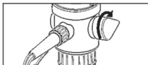
Make sure that the piston is moved completely to the bottom. When bubbles are no longer visible in the view glass the recirculation valve control should be set to titration (pointing toward the discharge tube) and the actual titration may begin.
