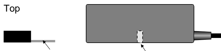
Figure 9: Correct orientation of the stirring drives MINI (left) and MICRO (right)
