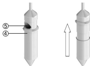
2. At the desired depth, pull back the instrument approx. 10 cm. Thereby, the sliding sleeve opens the filling opening.
