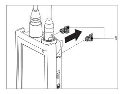
2 Push the electrode holder (1) into the recess (2) of the instrument.
