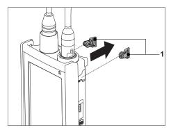
2 Push the meter base stabilizing unit (1) into the recesses (2) of the instrument.
