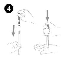
Put the sampling stick (A) back to the main body (B) and push it through all the way by putting the tip of the test tube (C) on a palm of hand or table. (Be careful not to get fingers caught when pushing it.)
