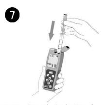
Insert the whole body of LuciPac Pen-AQUA into the measurement chamber of Lumitester and close the chamber's cover.
