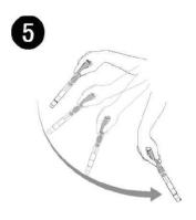
Shake the whole body of the LuciPac Pen-AQUA a few times so that the liquid in the capsule falls into the test tube (C).
