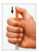
④ Shake the whole LuciPac Pen tube repeatedly so that all remaining liquid in the capsule falls into the reaction tube and dissolves the reagent in the tube.
