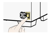
Push the On/Off switch on the appliance and disconnect power plug. This disconnects the appliance from the power supply at all poles.
