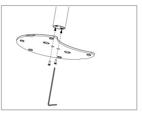
2 Then insert the foot of the meter to the arm base and shift the meter in the direction of the arrow to make the foot fit.
