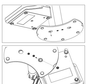
3 Use the lock screw to attach the meter to the base of the arm.
