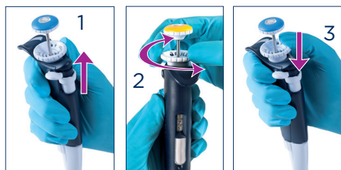
Figure 5 Volume unlock and unlock
