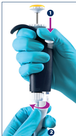
Figure 17 Removing the tip ejector
