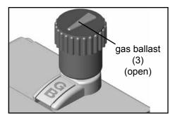
For **condensable vapors** (water vapor, solvents, etc.):
