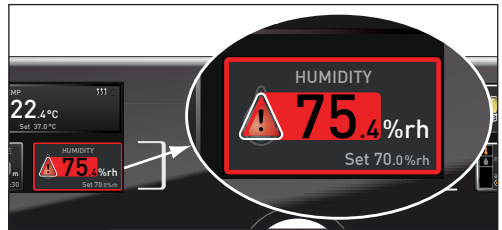
Fig. 22 Humidity monitoring triggered
