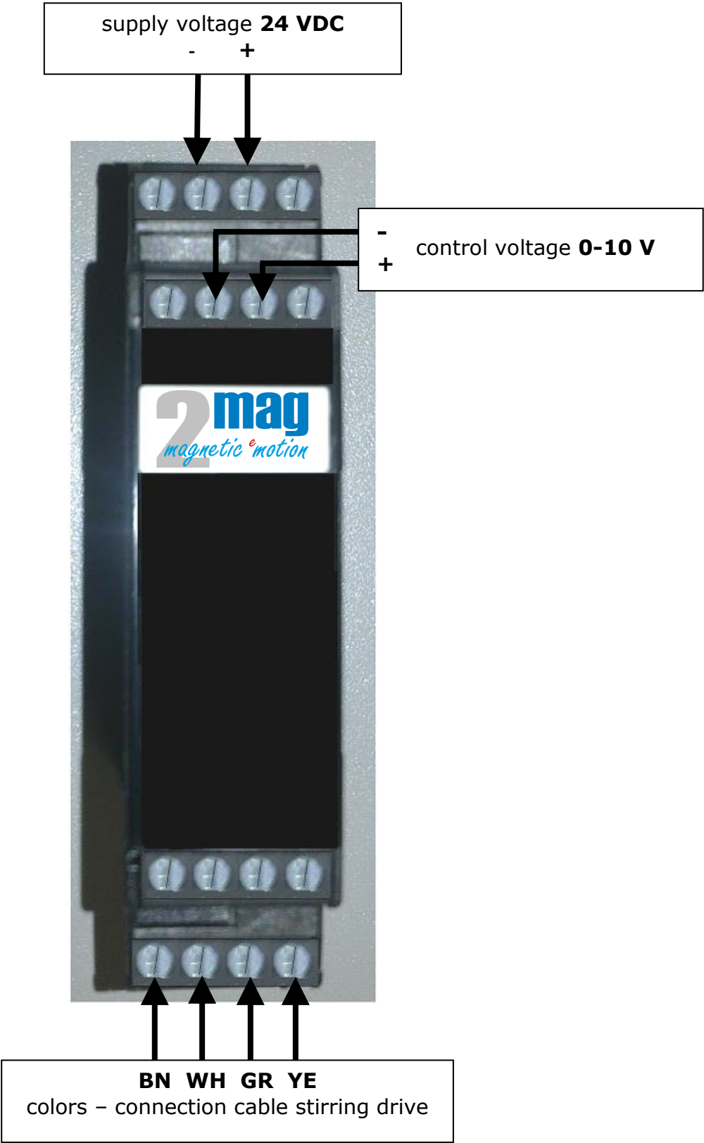
Image 8: Pin-assignment of MIXcontrol eco DINrail 0-10 volts
