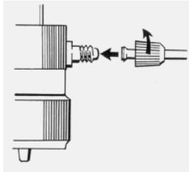
Screw the discharge tube set onto the thread adaptor of the PTFE valve block. Remove stopper cap from the discharge tube.
