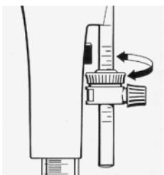
For calibrating purposes turn the screw of the fine adjustment. Turn downwards to increase the volume, turn upwards to decrease the volume.
