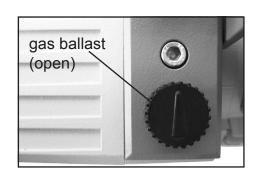
For **condensable vapors** (water vapor, solvents, etc.):
