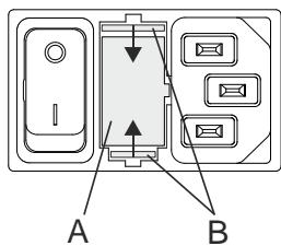
The fuse holder (A) with the mains input fuses is located next to the mains switch.
