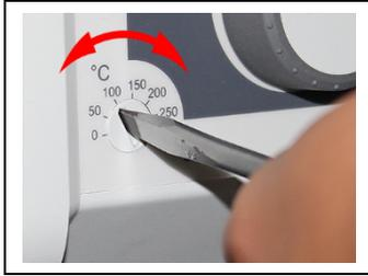
2. Use the screwdriver to set the high temperature cut-off.
