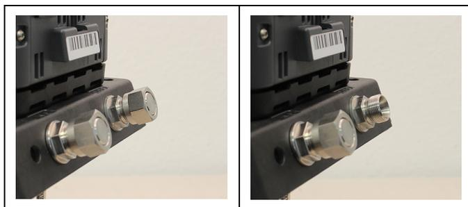
1. Remove the union nuts on the pump connections.
