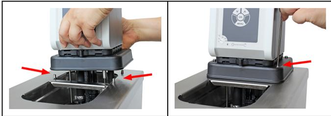
1. Carefully insert the circulator into the bath.
