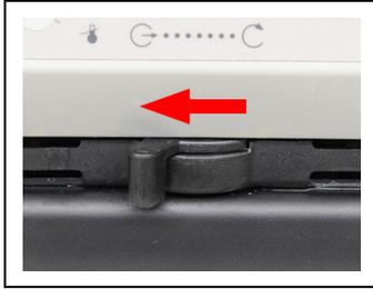
5. Set the flow direction lever to external circulation.
