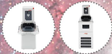
**Heating immersion circulator, open bath heating circulator,
