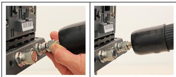
3. Screw the hoses onto the pump connections by hand.
