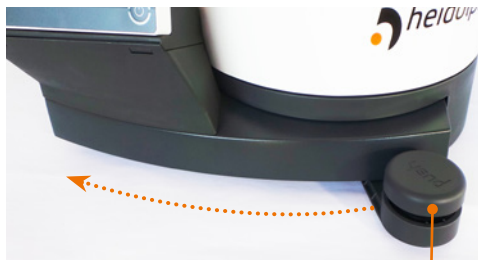
Manual lift lever: Lift position top
