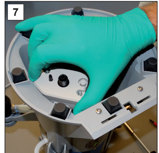
7. Pull out the VACUU-BUS plug downwards and remove the sensor.
