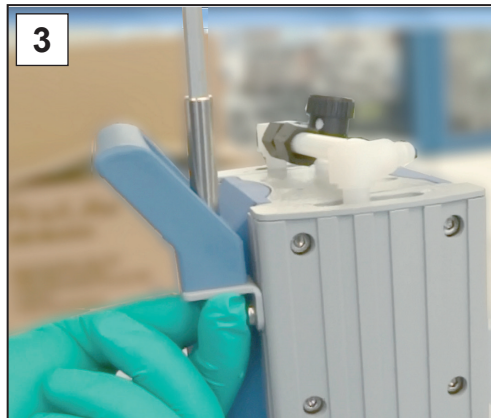
3. Loosen the screw connection from the handle; Allen key 5.
