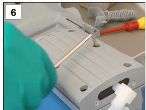
6. Unscrew the screw connections from the housing cover; Allen key 4.
