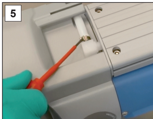
5. Open the hose clamp; flat-head screwdriver 1.
