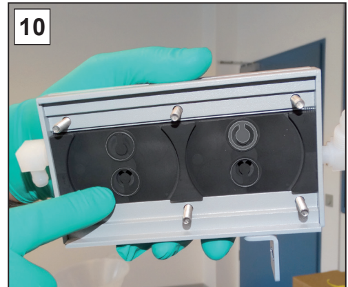
8. Check the housing cover for sticking valves and place the housing cover with the screw connections on the side.
