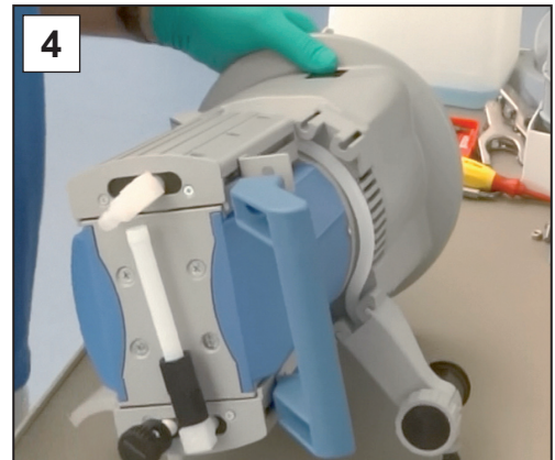
4. Lay the Pumping unit carefully on its side.
