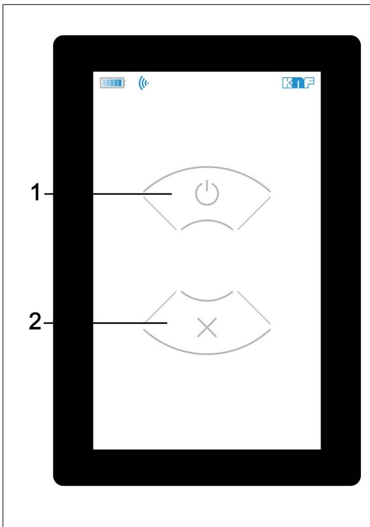
Fig.9: Switching the vacuum controller off
