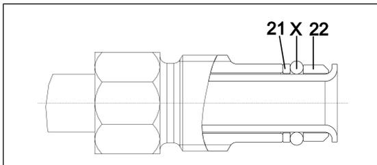
*Fig. 31: Correct position of O-ring*
