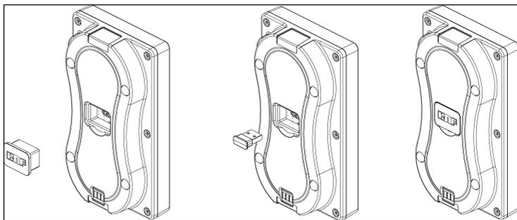
Fig. 10: Plugging Bluetooth stick into vacuum controller
