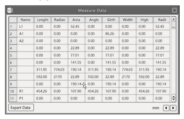
This table shows the details of the measuring elements drawn. By clicking on a line in the chart, the corresponding measuring element is activated and coloured yellow. By marking the measurement data in the chart, they can be changed.
