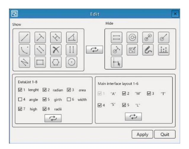
Measuring tool display: The left side shows the measuring instruments displayed on the user interface. The right side shows instruments that are not currently displayed. By marking two elements and clicking on the middle button, they can be exchanged. Click on "Apply" to apply the changes.
