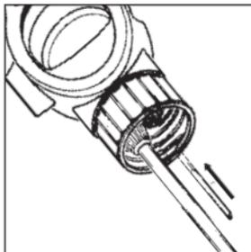
Insert the recirculation tube firmly into
