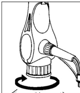
Screw the dispenser onto the reservoir bottle, either directly or with one of the enclosed adapters, depending on the bottle's thread size.
