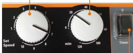
Select mode switch: continuous / timer
