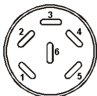
Figure 22: Pin configuration of the DIN socket(8) in the right lateral control panel
