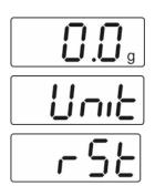
⇒ In weighing mode keep the **PRINT** key pressed until **[Unit]** appears.
