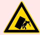
Danger of toppling over
