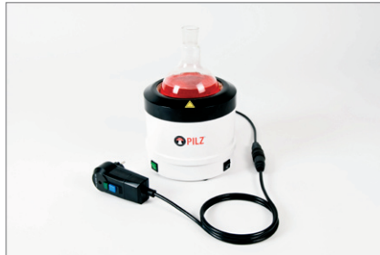
Fig. 2 – WHLG2 metal-cased heating mantle
