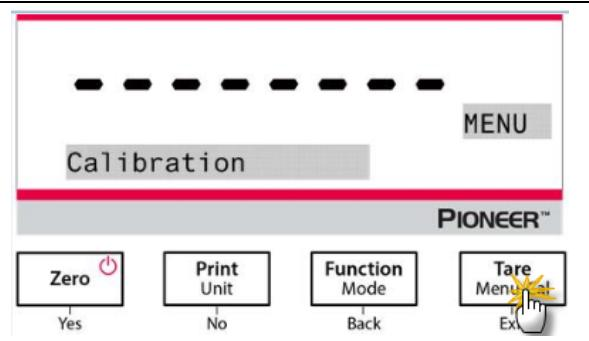
2. Press **Yes** to enter the Calibration Menu. To change the calibration mode, press **No** until Linearity Cal (linearity calibration) is displayed.
