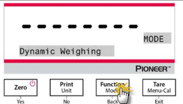
3. Press **Yes**, and then the message "Average time 10 s" will display with the numeral "10" flashing. Press **No** or **Back** to increase or decrease the value as desired.
