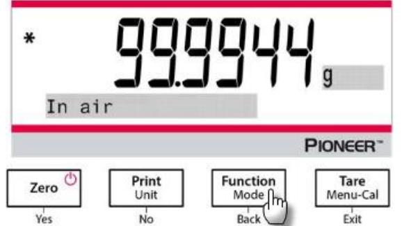
2. Weigh the sample submerged in the liquid using the balance and the density determination kit.
