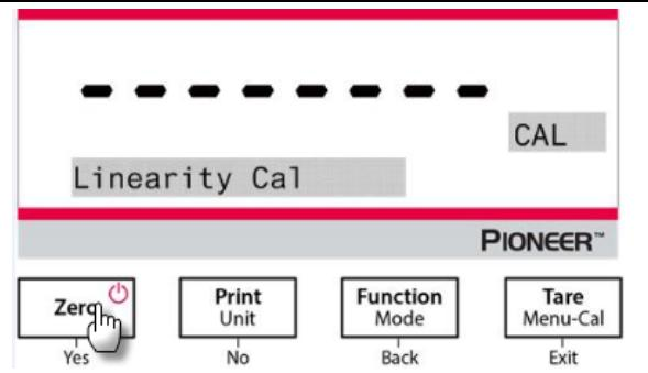
4. Calibration masses value will be shown in the screen. After the display shows "Place weights" and "50.0000 g", place weight(s) of 50 g on the pan for calibration.
