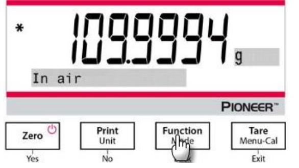
3. Weigh the oiled sample in the liquid with the balance and the density determination kit.
