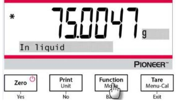
3. Press the **Function / Mode** button to get the density of the sample. After completion of the test, press the **Function / Mode** button to test a new sample.
