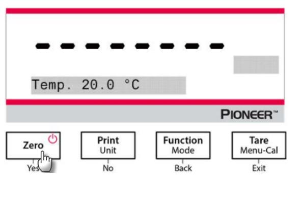
1. Weigh the sample in air using the balance and the density determination kit.
