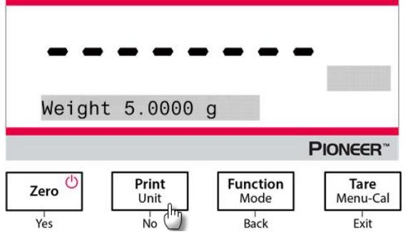
1. Weigh the oiled sample in the air with the balance and the density determination kit.
