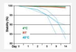
**Stability testing:** HPLC analysis of all four dNTPs following incubation periods of 1-14 days at different temperatures (4 °C - green; room temp.
