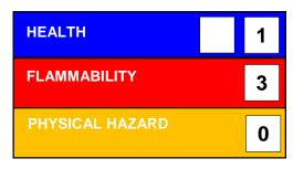
HMIS® ratings are based on a 0-4 rating scale, with 0 representing minimal hazards or risks, and 4 representing significant hazards or risks. The "\*" represents a chronic hazard, while the "/" represents the absence of a chronic hazard.
