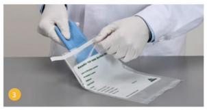
Put the swab into the sterile Twirl-Tie<sup>™</sup> bag and label bag with sample details. Always switch gloves between sampling sites.
