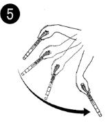
Shake the whole body of the LuciPac a few times so that the liquid in the capsule falls into the test tube (C).
