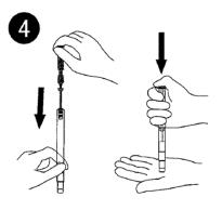
Put the sampling stick (A) back to the main body (B) and push it through all the way by putting the tip of the test tube (C) on a palm of hand or table. (Be careful not to get fingers caught when pushing it.)
