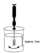
Soak sampling stick into water or other liquid samples, and shake it gently. Make sure any bubble don't remain in the comb of the sampling stick.
