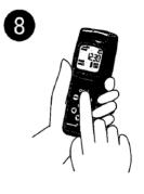
Press the "ENTER" key. Results are obtained in 10 seconds.
