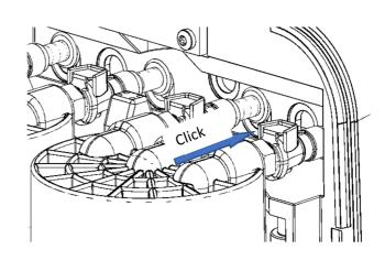
Then screw the sterile filter with its G1/4" thread into the outlet of the OptiFill dispenser (see figure).
