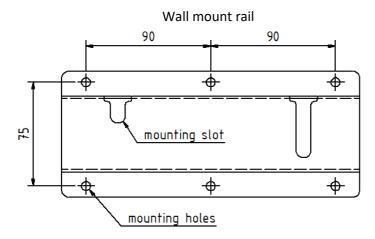
Then insert the dowels into the drilled holes and fasten the wall mounting rail to the wall with the screws so that the two mounting holes are facing upwards. Please note that the fastening material supplied with the wall holder is intended for installation in concrete and solid stone walls. If the wall holder is to be attached to a wall made of a different material, the fastening material must be replaced with a suitable one.
