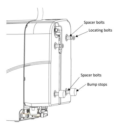
The next step is to attach the wall holder rail to the wall.
