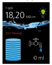
The system will now automatically start producing pure water and filling the tank. As soon as the maximum filling level of the tank is reached, the system automatically switches to circulation mode. Now empty a tank by pressing the withdrawal button and discard the water that has been withdrawn. The system is now ready for use.
